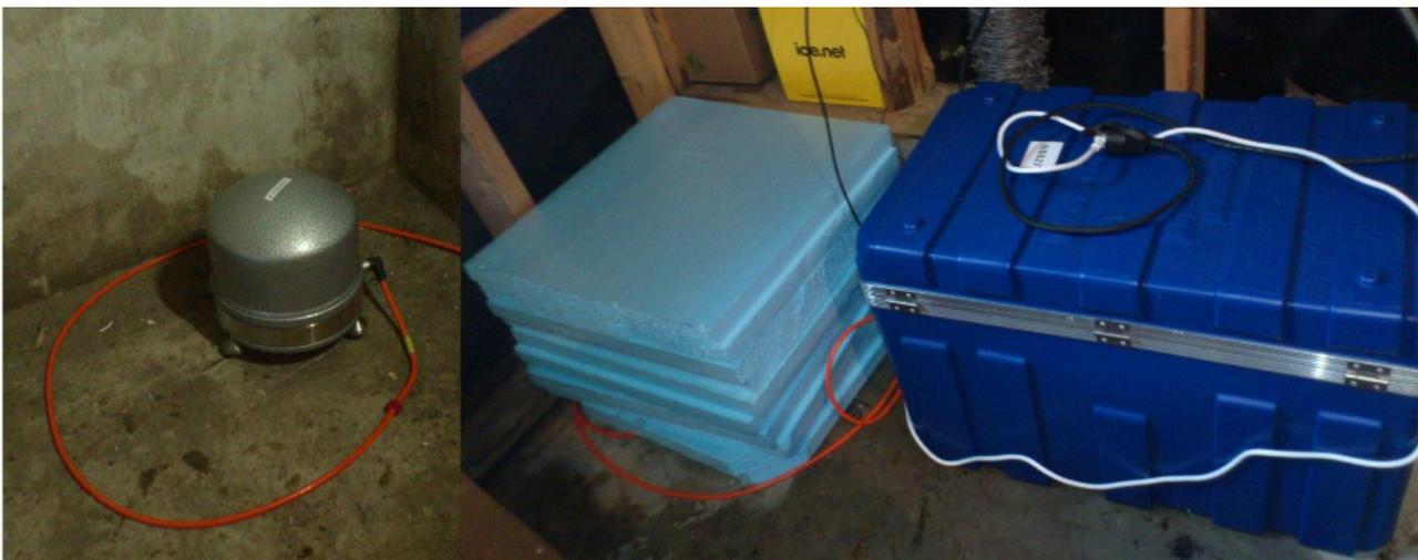
Examples of a seismometer (left) and the fully installed seismic station with insulation around the seismometer and a box containing additional instruments (right).
